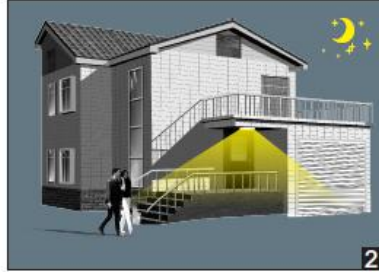
2 With insufficient ambient light, the sensor switches on the lamp when motion is detected.
